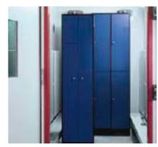
Salt spraying chamber with two lockers which are being tested as a complete product according to DIN 50021 at C+P.
