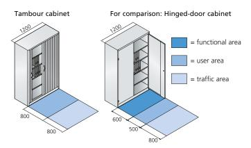
Sample visualization of the functional floor space required by space-saving cabinet types
