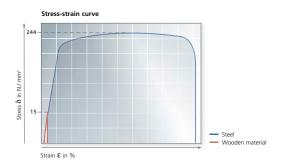
The stress-strain curve describes how easily a material can be distorted and when the material will fail, i.e. break. You can see that, in comparison to wood, steel is very difficult to distort, can withstand extremely strong forces and also provides a certain safety scope even in the critical range thanks to its plastic behavior.
