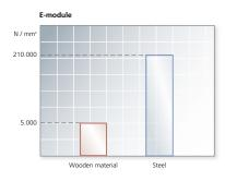
The "elasticity module" defines the ratio of the force required to cause a distortion and the distortion it causes. In other words: how much force must I apply to stretch a material? The diagram shows that steel is unbeatable as a material in terms of stability and elasticity.
