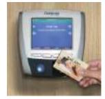
Online locking system with central info terminal, with PIN or transponder/data carrier
